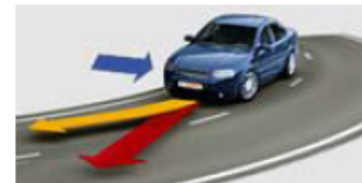
Figure 46. ESC is active all the time. It recognizes critical situations before the driver can and intervenes independently. From (Bosch 2008).
